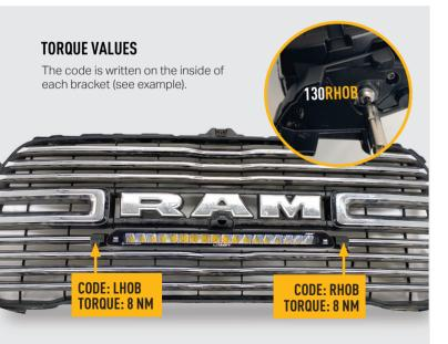
**INSTALLATION PROCESS** - Linear-18 shown for illustration purposes. Install should be completed with the grille left on the vehicle.
