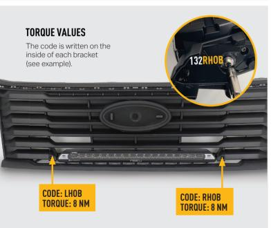
**INSTALLATION PROCESS** - Linear-18 shown for illustration purposes. Install should be completed with the grille left on the vehicle.
