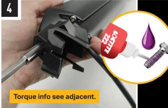
Please use a thread seal compound (i.e. Loctite 222) to protect the . lamp fastener from binding over time.
