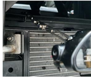
Position the brackets as shown. Drill through the bumper beam (5mm drill) and rivet the brackets to the bumper beam. 4 rivets per bracket.
