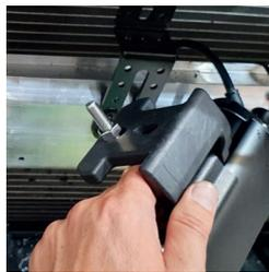
Use extra nut as spacer as shown before mounting the centre mounts to the bumper beam brackets.
