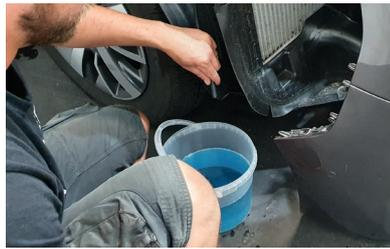
Undo the tube for the headlight washers and catch screen wash in bucket then bumper can be removed .
