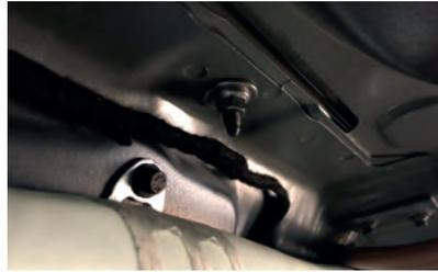
You can now access the 5x 10mm bolts (per roof rail) to remove the roof rails, remove the bolts:
