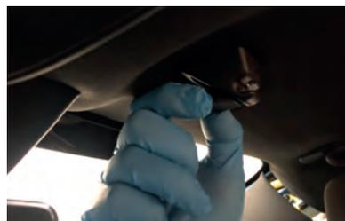
On both sides of the vehicle, remove the retaining clip and then remove the sun visor hook.
