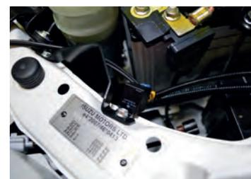
Install the relay and connect the live and earth to the battery, the high beam trigger is taken from the back of the headlight.
