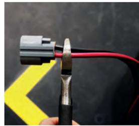
Remove Switch from the crimp terminals and cut of the lamp connector from the wiring harness.
