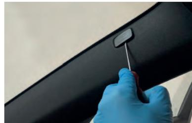
Remove 'A' pillar bolt cover and undo 8mm bolt.
