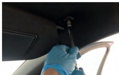
Undo the 2x 7mm bolts and unplug the sunvisors.
