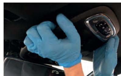
Pull the centre of the interior light panel down and unplug and remove.
