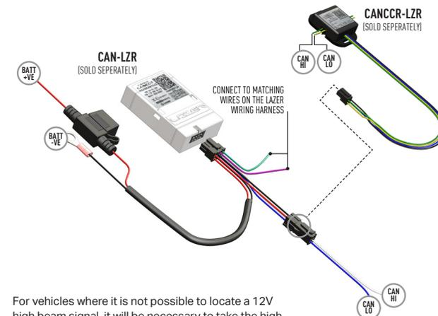
For vehicles where it is not possible to locate a 12V high beam signal, it will be necessary to take the high beam signal from the vehicle's CAN system. For vehicle specific CAN instructions, please download the "CANMB Connect" App.
