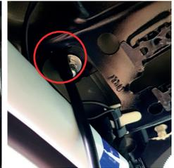
8. Mount the light bar using the supplied spacers, washers and 70mm bolts.
