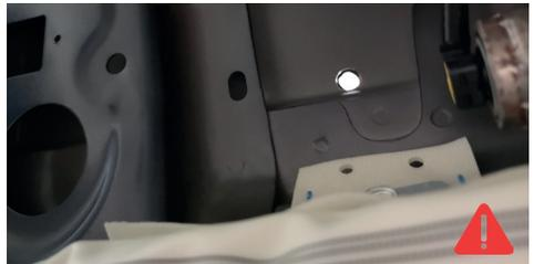
3. Drill a 8mm hole 90mm from the top of the **left** roof rail and insert 2nd cable grommet.
