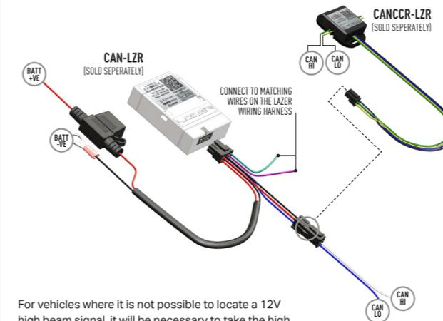
For vehicles where it is not possible to locate a 12V high beam signal, it will be necessary to take the high beam signal from the vehicle's CAN system. For vehicle specific CAN instructions, please download the "CANMS Connect" App.
