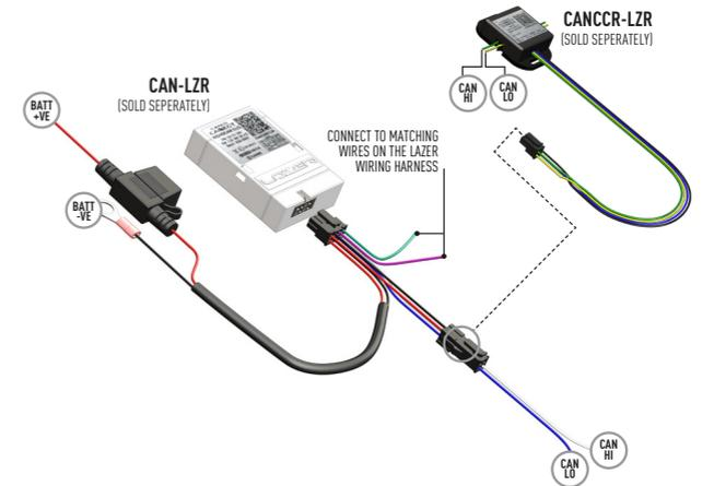
For vehicles where it is not possible to locate a 12V high beam signal, it will be necessary to take the high beam signal from the vehicle's CAN system. For vehicle specific CAN instructions, please download the "CANM8 Connect" App.
