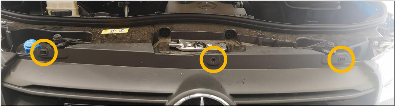
Remove the 3x Screws holding in the grille, and remove the front grille.
