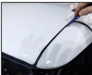
Alternatively, it may be possible to run the cable up the outside of the 'A' pillar or windscreen, without having to drill a hole. If this is the case, route the cable as desired and plug the lamp in (be sure to secure any cables).
