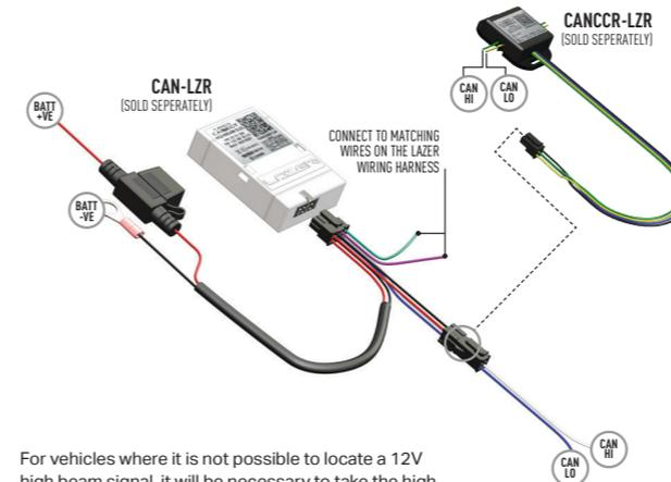
For vehicles where it is not possible to locate a 12V high beam signal, it will be necessary to take the high beam signal from the vehicle's CAN system. For vehicle specific CAN instructions, please download the "CANM8 Connect" App.
