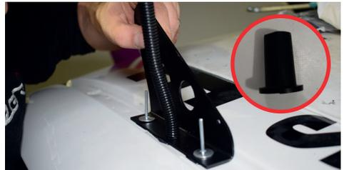
6. Add the rivets and using a rivet gun secure the bracket to the roof. Repeat step for right-hand side (minus cable entry).
