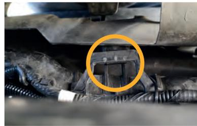
Pull top centre of bumper up and unclip the retaining clips on both sides of the vehicle.
