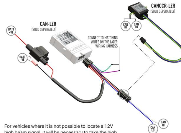
For vehicles where it is not possible to locate a 12V high beam signal, it will be necessary to take the high beam signal from the vehicle's CAN system. For vehicle specific CAN instructions, please download the "CANM8 Connect" App.
