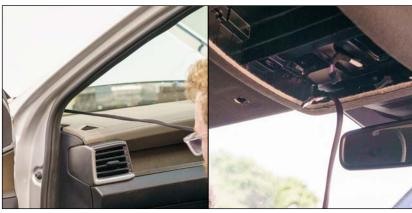
With the wire inside, run it up the A-pillar and along the roof to the roof console opening, securing to existing wiring with cable ties where possible.
