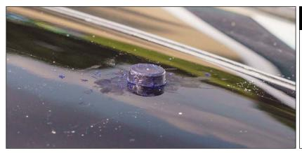
Fit grommet to the roof, ensuring the roof skin is in the ridge all the way around on the inside to make a complete seal.
