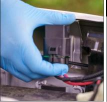
Mount the relay holder in suitable place within the engine bay.
