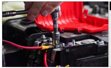
Connect 12v positive lead to the relay to one of the accessory power points on the battery.
