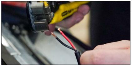
Strip back wires on the pod and the vehicle side wiring loom.
