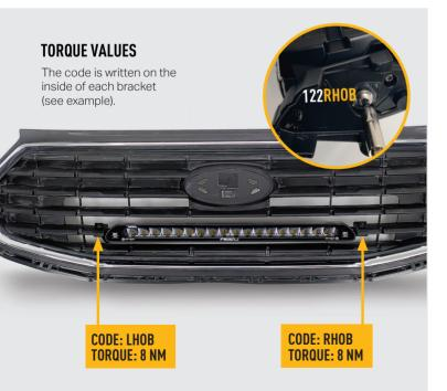
INSTALLATION PROCESS - Linear-18 shown for illustration purposes. Install should be completed with the grille left on the vehicle.
