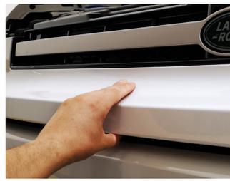
Loosen the lower section of the grille and remove the grille surround.
