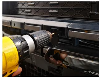
Make sure the lamp is level and drill 5mm hole for the inboard brackets to be riveted into place.
