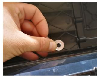
Rivet the bracket into place. Install the included washer behind the rivet to spread the weight of the lamp.
