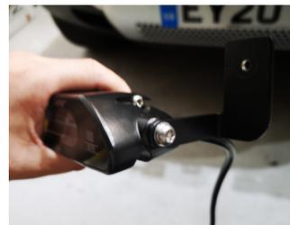
Temporarily install the inboard brackets onto the lamps.
