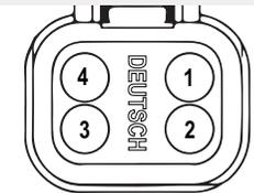
Vehicle side will require the a DT06-4S Deutsch Connector.
