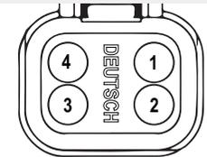
Vehicle side will require the a DT06-4S Deutsch Connector.
