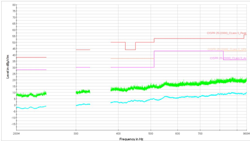
Figure 29. Ambient measurement. From 200 to 1000MHz. Vertical Polarization. Peak and Average measurement.
