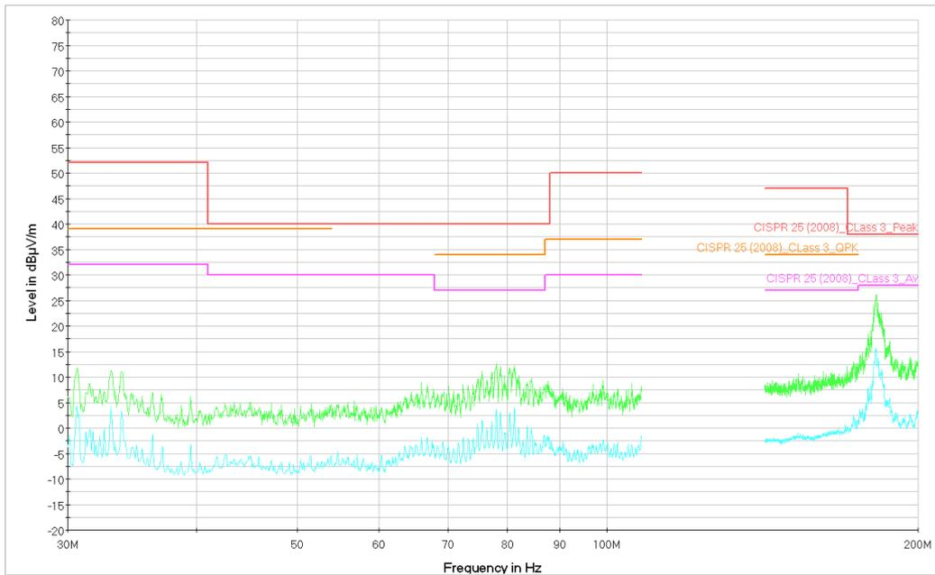
Figure 41. Sample 2. From 30 to 200MHz. Vertical Polarization. Peak and Average measurement.
