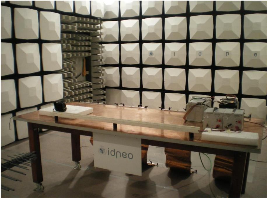
Figure 23. . RE Test. Test Setup from 200MHz to 1000MHz. WL80 G2
