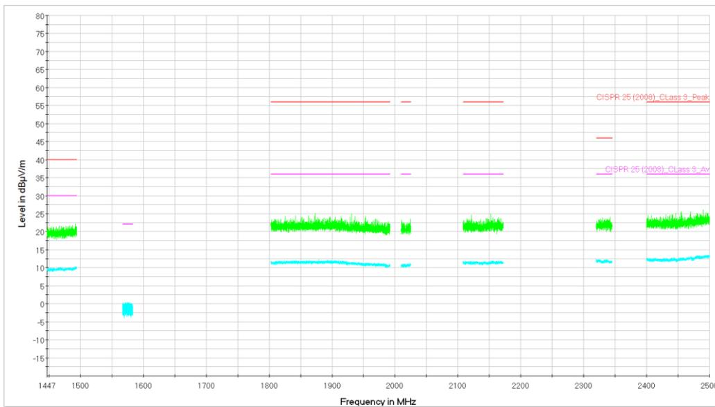
Figure 30. Ambient measurement. From 1000 to 2500MHz. Horizontal Polarization. Peak and Average measurement.
