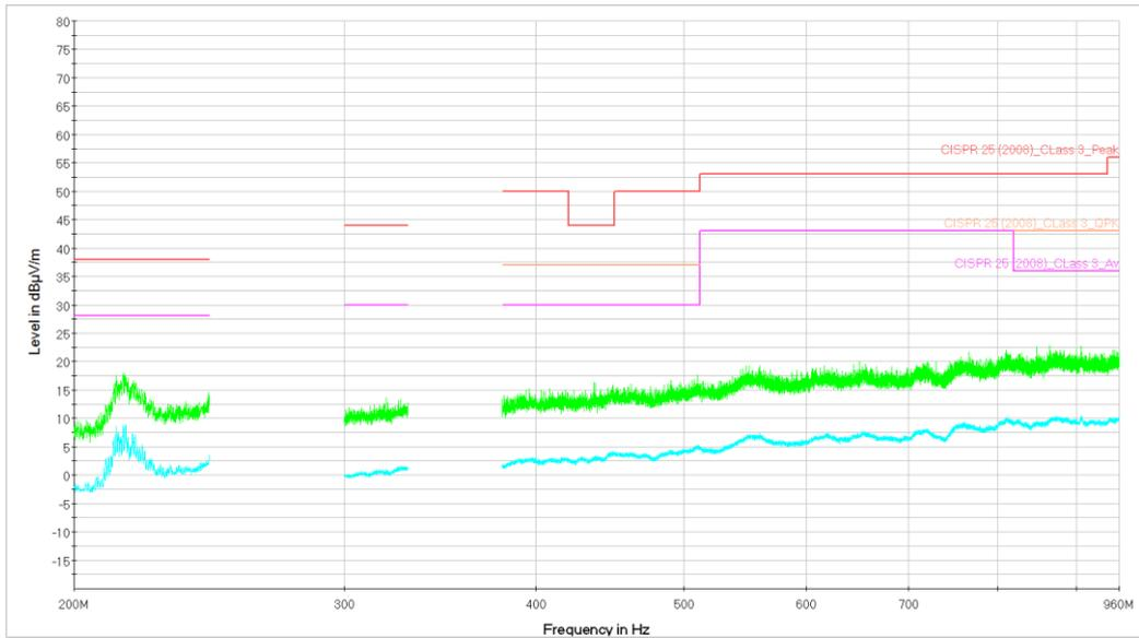
Figure 35. Sample 1. From 200 to 1000MHz. Horizontal Polarization. Peak and Average measurement.
