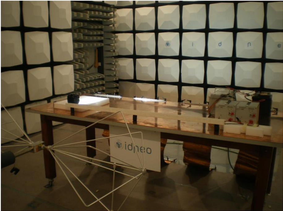
Figure 18. . RE Test. Test Setup from 30MHz to 200MHz. WL45 G2
