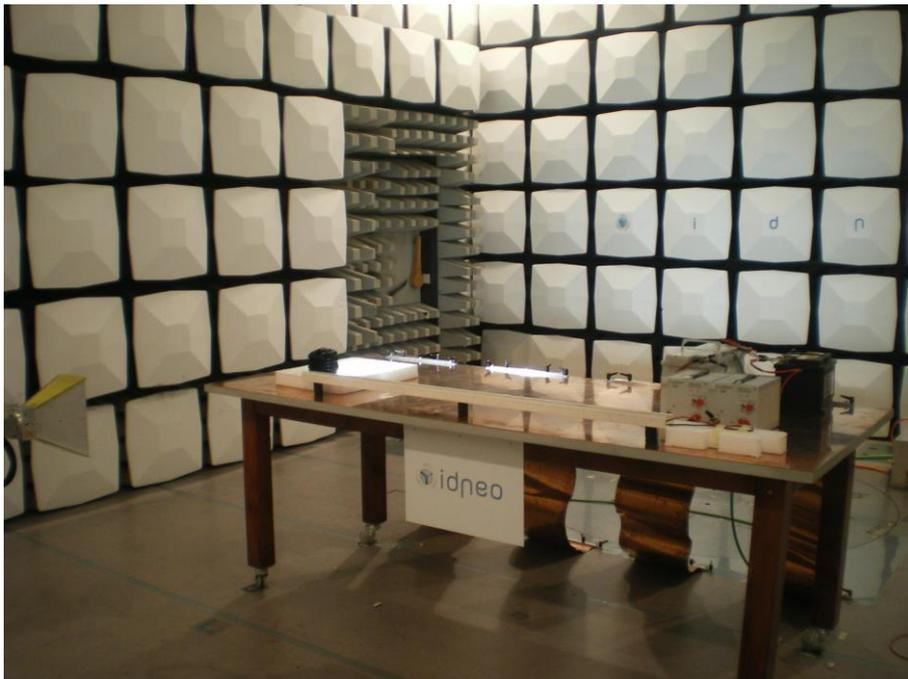
Figure 20. . RE Test. Test Setup from 1000MHz to 2500MHz. WL45 G2
