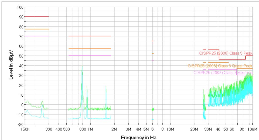
Figure 9. Test measurement. Sample 1. GND Line. From 150kHz to 108MHz. Peak and Average measurements.
