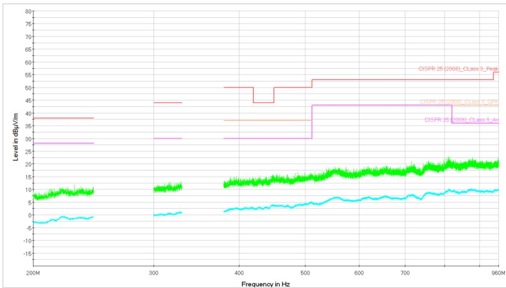
Figure 28. Ambient measurement. From 200 to 1000MHz. Horizontal Polarization. Peak and Average measurement.
