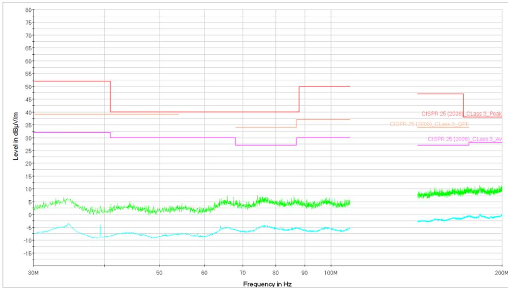
Figure 27. Ambient measurement. From 30 to 200MHz. Vertical Polarization. Peak and Average measurement.
