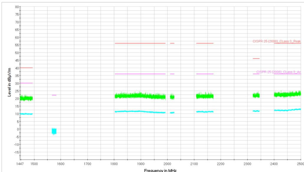
Figure 38. Sample 1. From 1000 to 2500MHz. Vertical Polarization. Peak and Average measurement.
