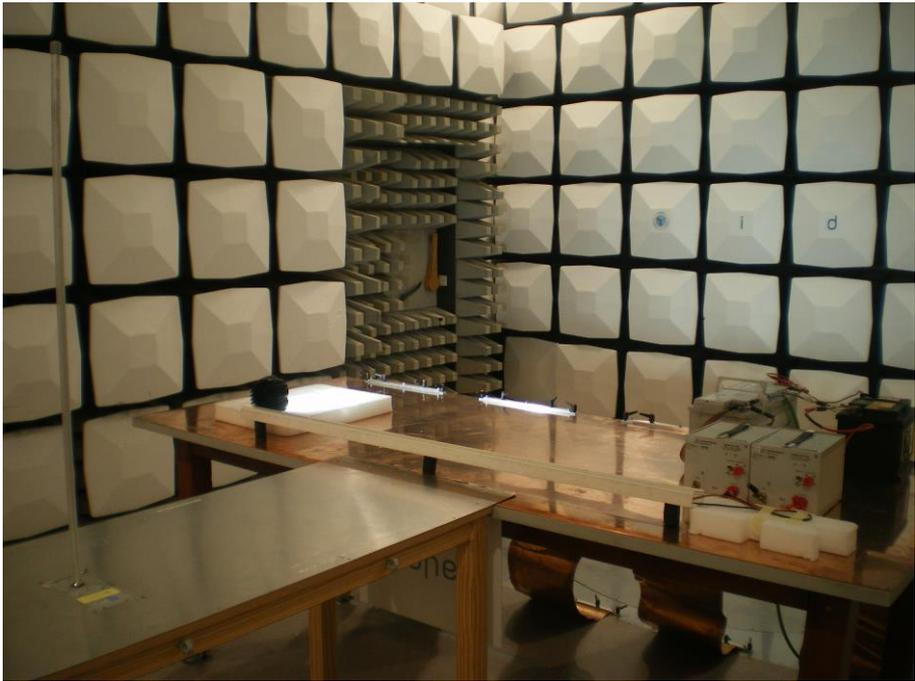
Figure 17. RE Test. Test Setup from 100kHz to 30MHz. WL45 G2
