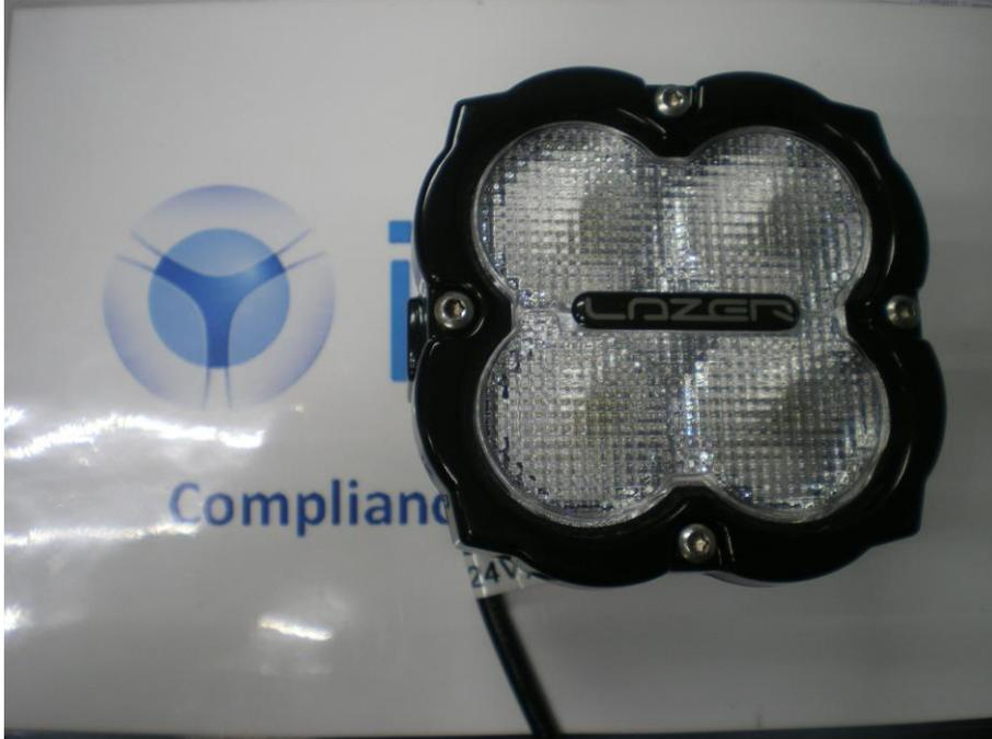
Figure 1. Sample under test WL45 G2 Lamp (Lens picture is not according to the production level).
