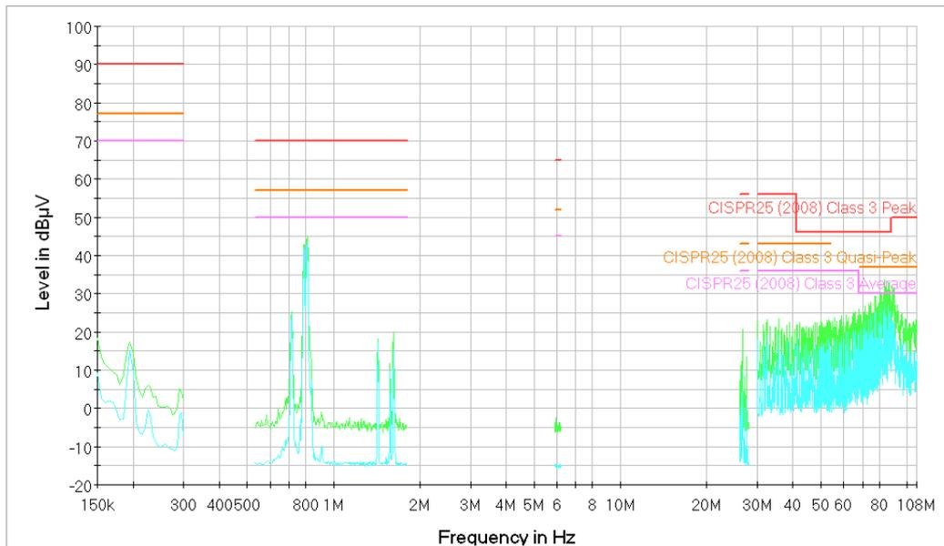
Figure 12. Test measurement. Sample 2. VCC Line. From 150kHz to 108MHz. Peak and Average measurements.
