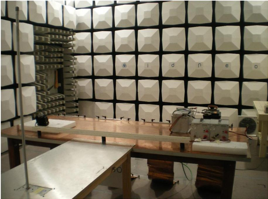
Figure 21. RE Test. Test Setup from 100kHz to 30MHz. WL80 G2
