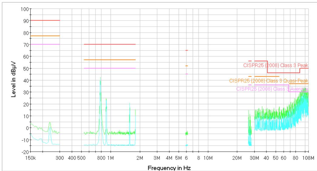
Figure 10. Test measurement. Sample 1. VCC Line. From 150kHz to 108MHz. Peak and Average measurements.
