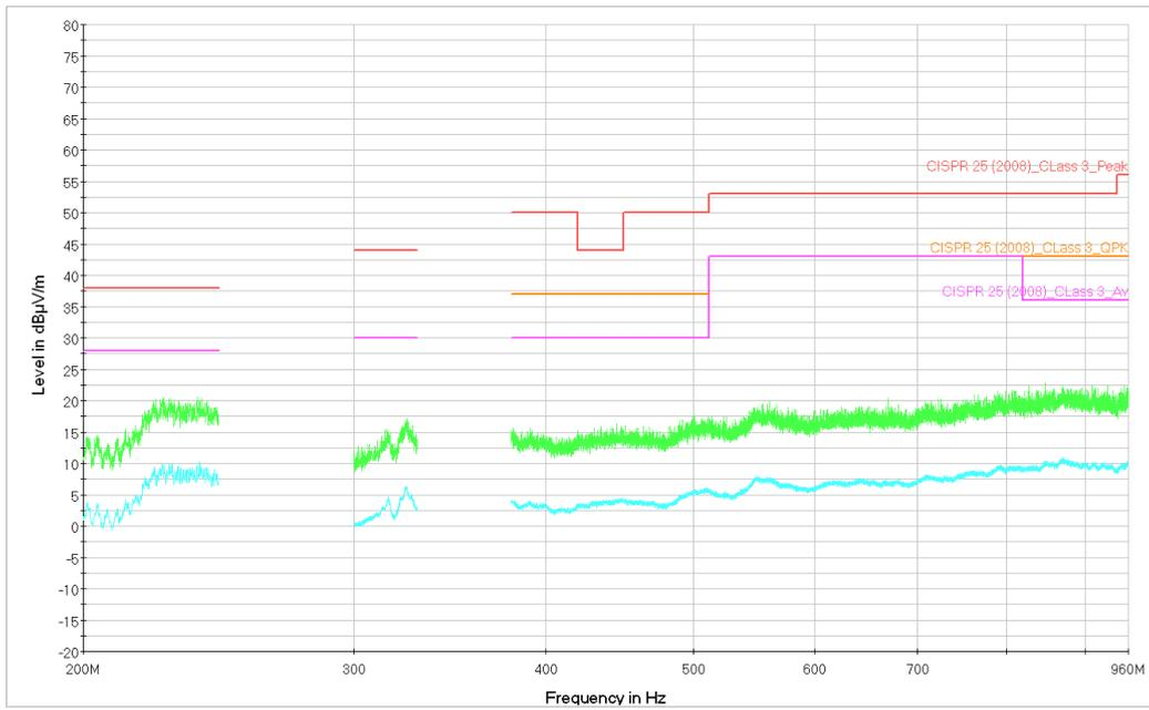
Figure 43. Sample 2. From 200 to 1000MHz. Vertical Polarization. Peak and Average measurement.
