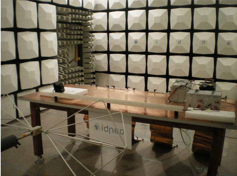
Figure 22. . RE Test. Test Setup from 30MHz to 200MHz. WL80 G2
