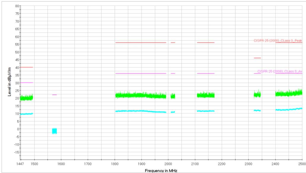
Figure 37. Sample 1. From 1000 to 2500MHz. Horizontal Polarization. Peak and Average measurement.
