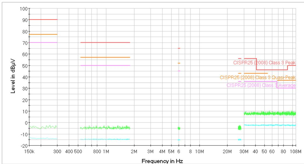
Figure 8. Ambient measurement. VCC Line. From 150kHz to 108MHz. Peak and Average measurement.
