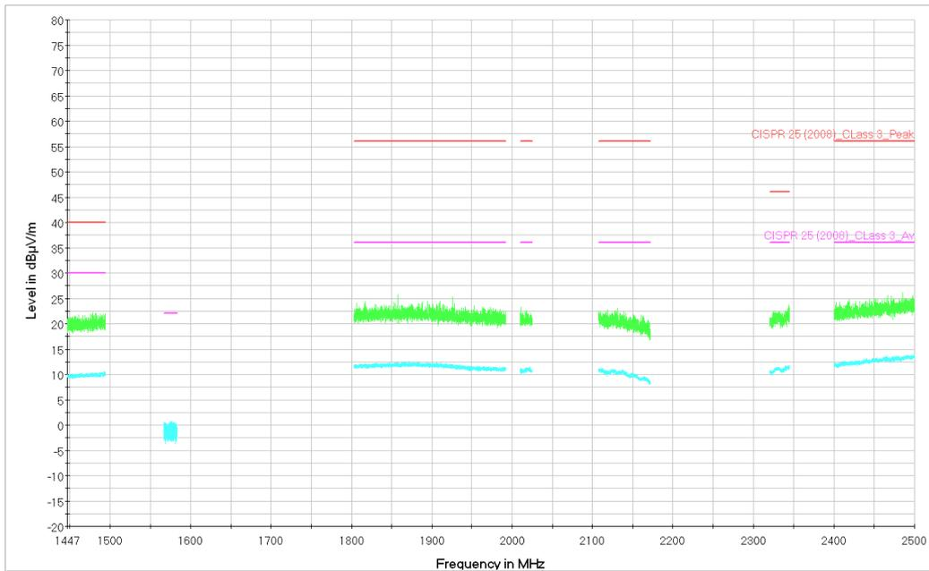
Figure 44. Sample 2. From 1000 to 2500MHz. Horizontal Polarization. Peak and Average measurement.
