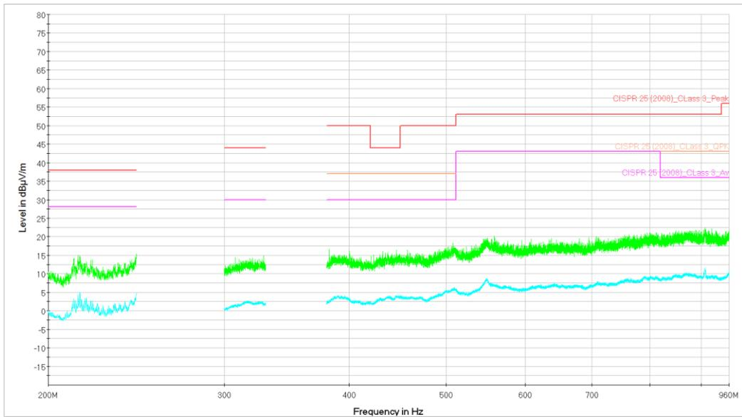
Figure 36. Sample 1. From 200 to 1000MHz. Vertical Polarization. Peak and Average measurement.
