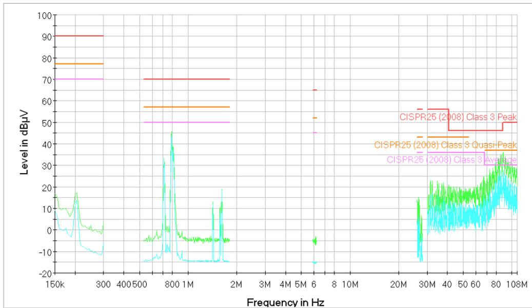
Figure 11. Test measurement. Sample 2. GND Line. From 150kHz to 108MHz. Peak and Average measurements.
