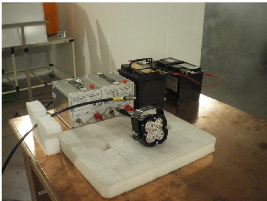
Figure 6. CE Test. Test Setup applied for WL80 G2 lamp.
