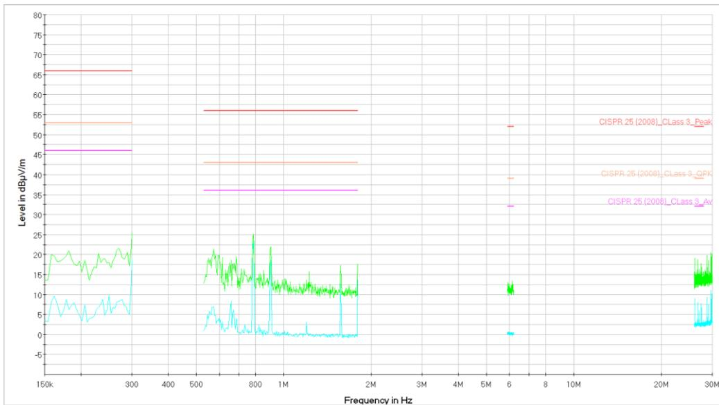
Figure 32. Sample 1. From 100kHz to 30MHz. Peak and Average measurements.
