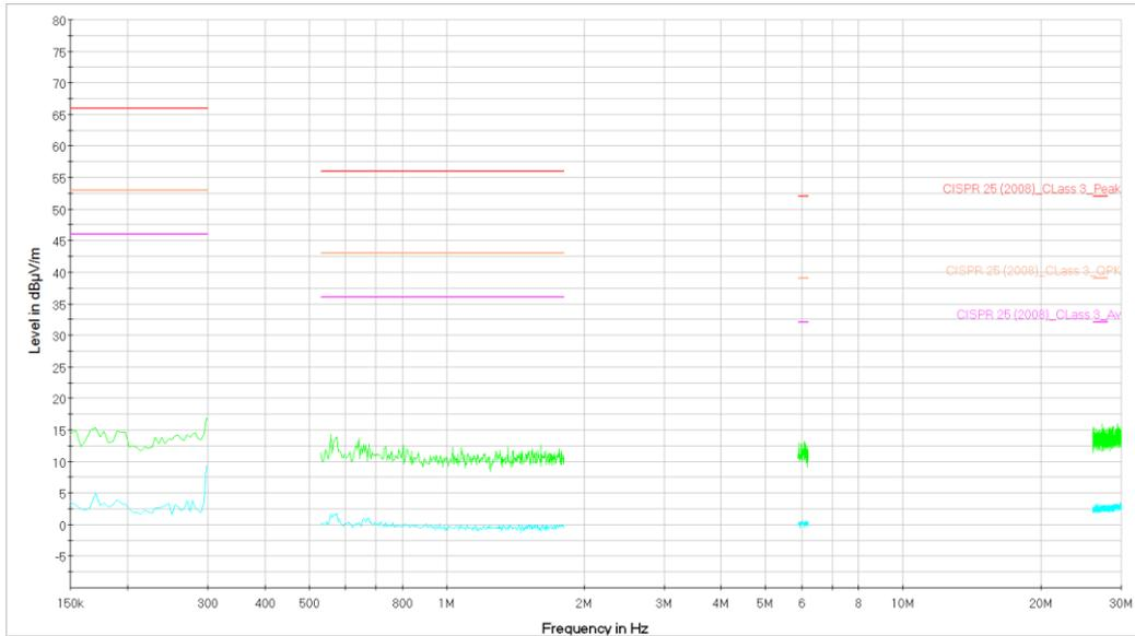
Figure 25. Ambient measurement. From 150kHz to 30MHz. Peak and Average measurement.
