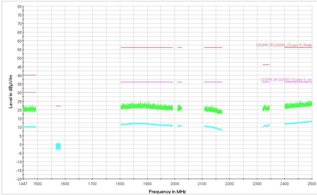
Figure 45. Sample 2. From 1000 to 2500MHz. Vertical Polarization. Peak and Average measurement.
