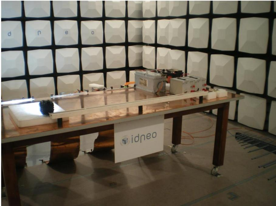
Figure 19. . RE Test. Test Setup from 200MHz to 1000MHz. WL45 G2
