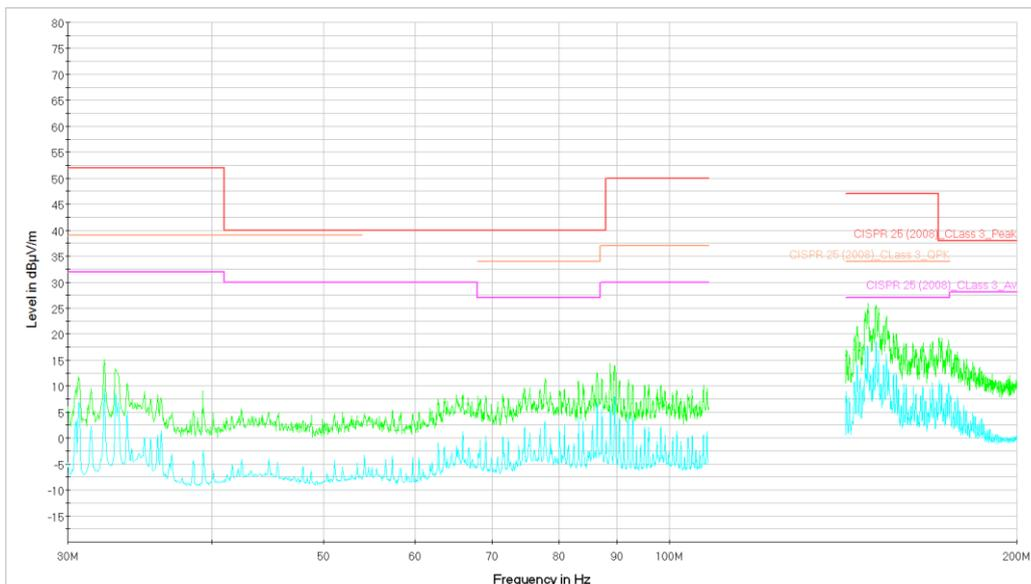
Figure 34. Sample 1. From 30 to 200MHz. Vertical Polarization. Peak and Average measurement.
