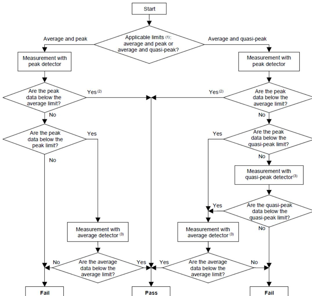
Figure 3. Acceptance Criteria Flow Chart – Radiated and Conducted Emissions.
