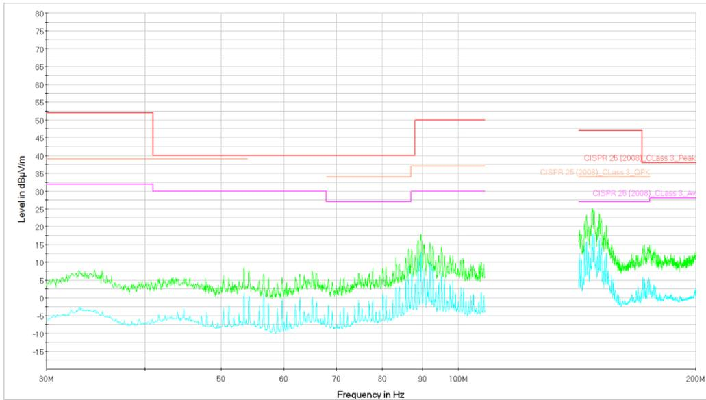
Figure 33. Sample 1. From 30 to 200MHz. Horizontal Polarization. Peak and Average measurement.
