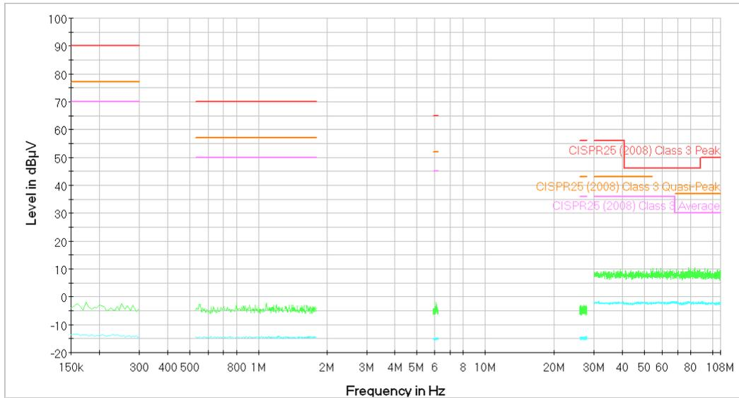
Figure 7. Ambient measurement. GND Line. From 150kHz to 108MHz. Peak and Average measurement.
