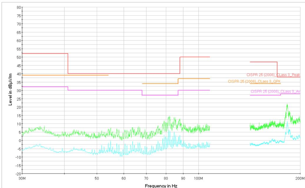
Figure 40. Sample 2. From 30 to 200MHz. Horizontal Polarization. Peak and Average measurement.
