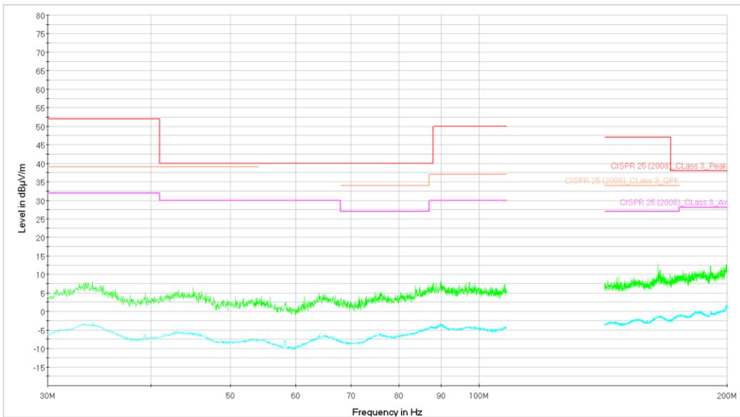
Figure 26. Ambient measurement. From 30 to 200MHz. Horizontal Polarization. Peak and Average measurement.
