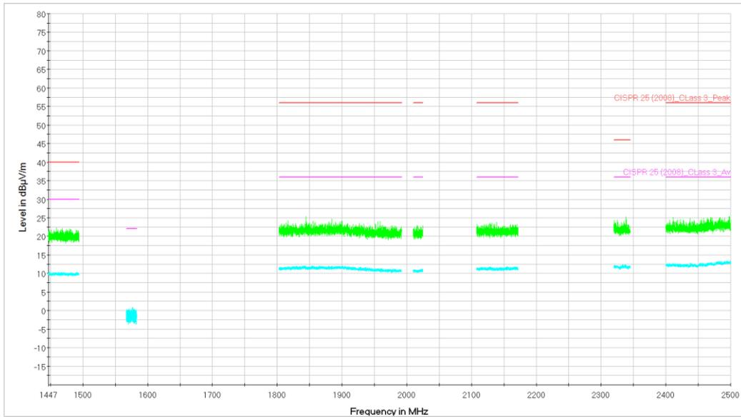
Figure 31. Ambient measurement. From 1000 to 2500MHz. Vertical Polarization. Peak and Average measurement.
