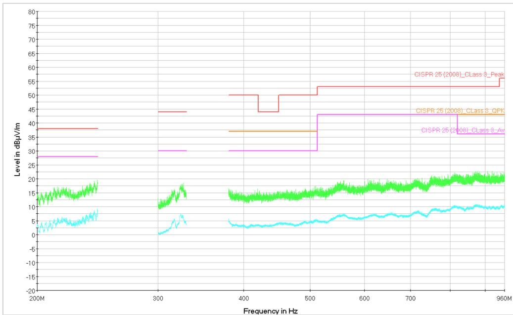
Figure 42. Sample 2. From 200 to 1000MHz. Horizontal Polarization. Peak and Average measurement.
