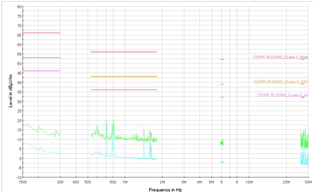
Figure 39. Sample 2. From 100kHz to 30MHz. Peak and Average measurements.
