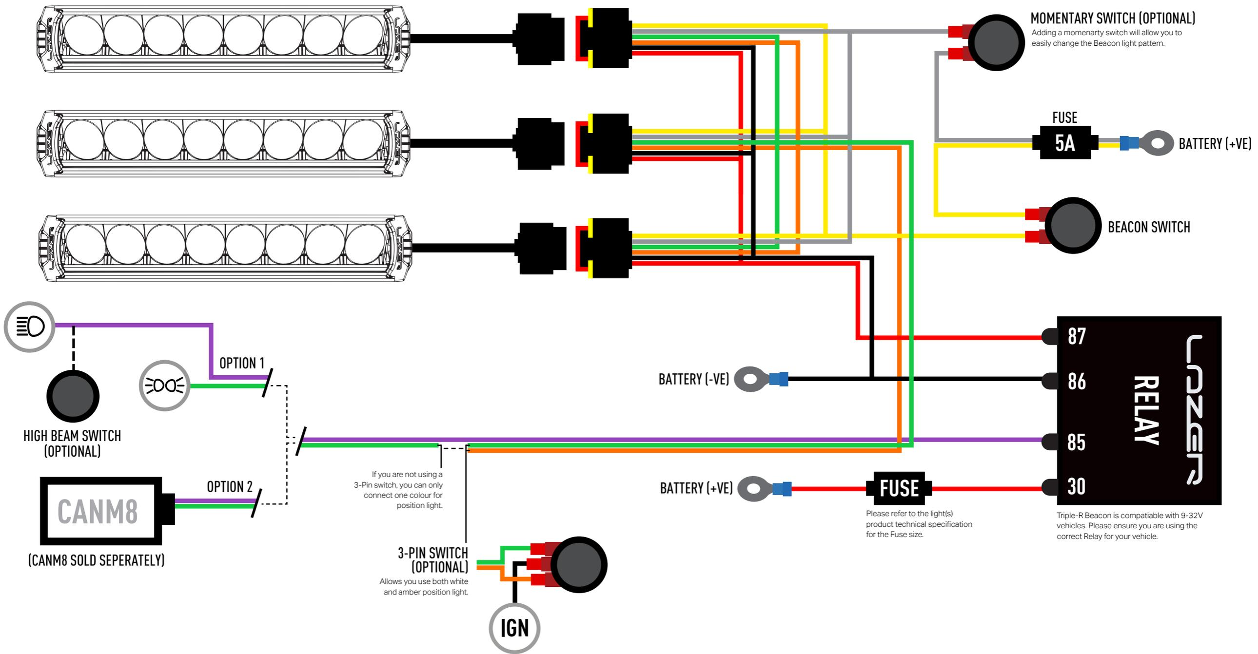
Triple-R Beacon is compatible with 9-32V vehicles. Please ensure you are using the correct Relay for your vehicle.
