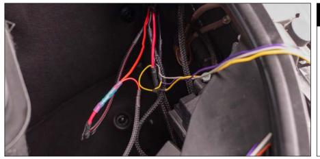
Connect the wire back to the relay power lead. In our case, we are also using CANNY so have connected its power here also. Ground for the relay and canny are connected to the jump start negative post.
