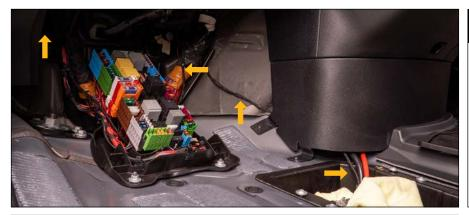
Run the wire out to the engine bay, following as much original wiring as possible.
