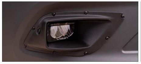
Repeat for the other x6 holes, being careful to not over torque the screw in the soft plastic bumper.
