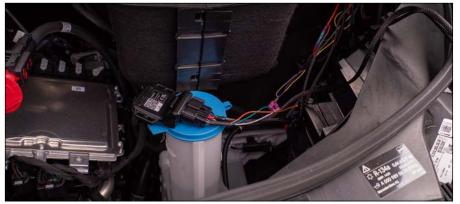
Connect CANNY to the harness and find suitable place to mount the device.
