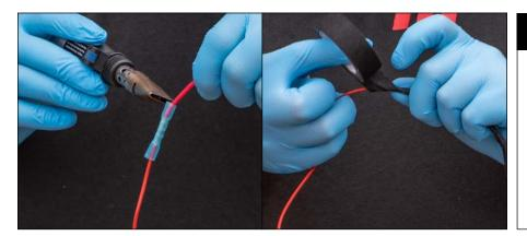
Heatshrink the crimp and loom tape up the wire.
