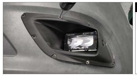
Place the bezel into the fog pocket and visually align to shape, taking care to ensure the lamp is horizontal.
