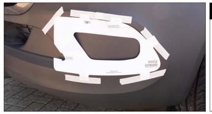
Attach the templates to the bumper using tape.
