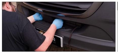
Pass the right hand wire across the front of the vehicle – securing wires as you go.
