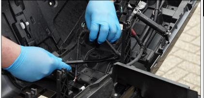
Move the wiring harness out the way of cutting area (where you have masked on the front).
