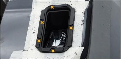
Drill the x5 mounting holes using a 3mm drill bit.
