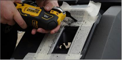
Using a multi tool, cut out the rectangle you have drawn on, using the corner holes to help start.
