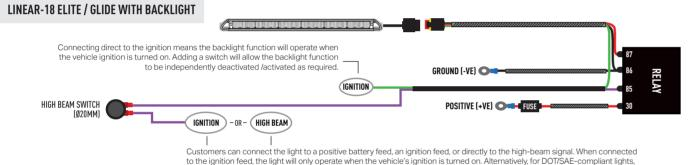
to the ignition feed, the light will only operate when the vehicle's ignition is turned on. Alternatively, for DOT/SAE-compliant connecting directly to the high-beam signal will allow the light to operate in sync with your vehicle's high beams.
