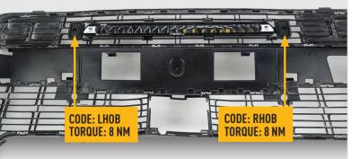
INSTALLATION PROCESS - Linear-18 shown for illustration purposes. Install should be completed with the grille left on the vehicle.
