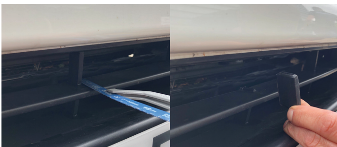
4. Using cutters or a blade, remove the upper centre grille vein as shown.
