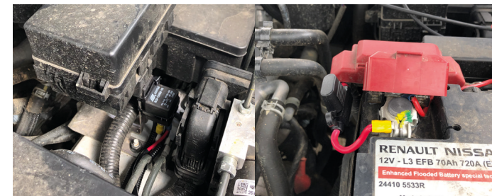
3. Install Relay close to the battery and connect the live and earth feed to battery. Connect signal wire according to preferred method (splice or switch).
