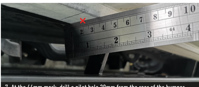
7. At the 66mm mark, drill a pilot hole 20mm from the rear of the bumper towards the front.
