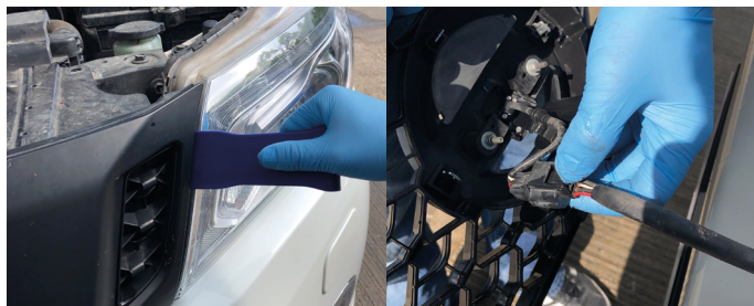
2. Unclip grille sides using a plastic trim removal tool. If vehicle has a front camera, this will need to be unplugged to remove grille.
