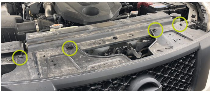
1. Remove trim clips that are located under the bonnet for the front grille.
